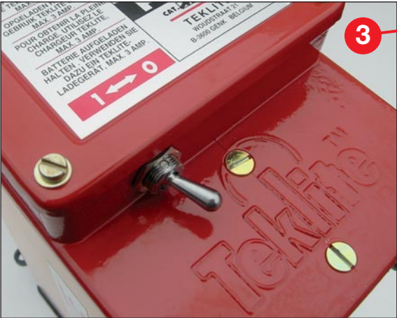
Built-in circuit board with integrated ON/OFF switch.
