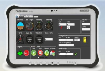
The remote deck panel is designed for the real time monitoring of USV's navigation, communication and driving system statuses. The panel serves as a constant checkpoint for the operator, providing him with full situational awareness and secure remote control.
